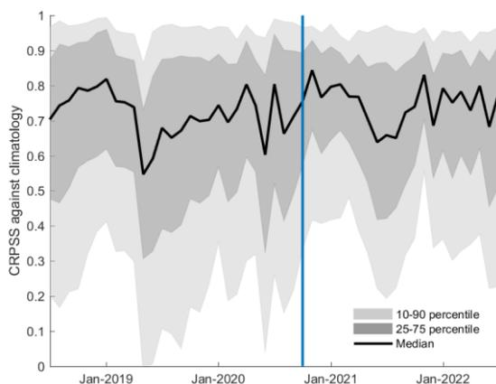
**Figure 4.** Monthly means of CRPSS the for lead-time 5 days for all the major river points in Europe with ECMWF ENS as forcing. Reference forecast was climatology. The skill is largest during the winter months, when there is less variation in the flow in large parts of Europe. The blue line indicates the release of EFAS 4.0.
