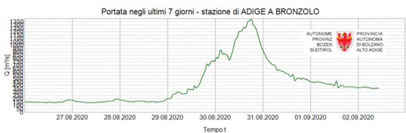
Figure 13: Observed discharge recorded at Bronzolo gauging station (courtesy of Provincia Autonoma di Bolzano Alto Adige). EFAS version 4.0 forecasts
